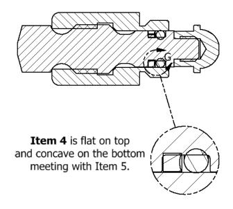
NOTE: The orientation of the back-up ring is important. The concave face must point towards the O-Ring.
