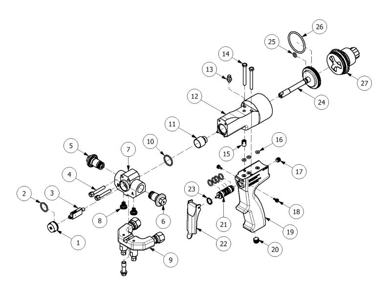
**NOTE:** WHEN ASSEMBLING BE SURE TO APPLY GREASE TO **ALL** O-RINGS. THIS ENSURES GOOD PERFORMANCE AND REDUCES RISK OF GUN MALFUNCTION.
