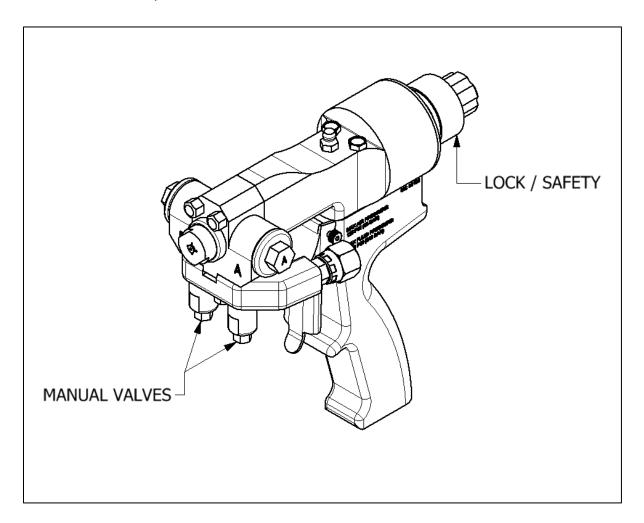
WARNING! Before proceeding with any maintenance work on the AP-3 Gun, trigger the gun to remove internal material pressure, ensure the Manual Valves are CLOSED, ensure the Gun Lock is in the LOCKED position, and SHUT OFF/DISCONNECT the air supply. It is recommended to remove the Gun from the Coupling Block.
