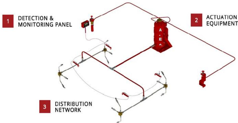
**Figure 3 – Typical Dry Powder Suppression System used for Vehicles.**
